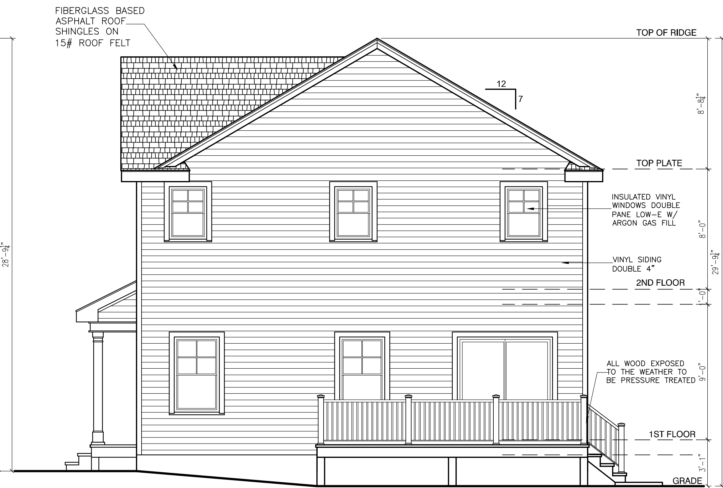
RIGHT SIDE ELEVATION SCALE 1/4" = 1'-0"
