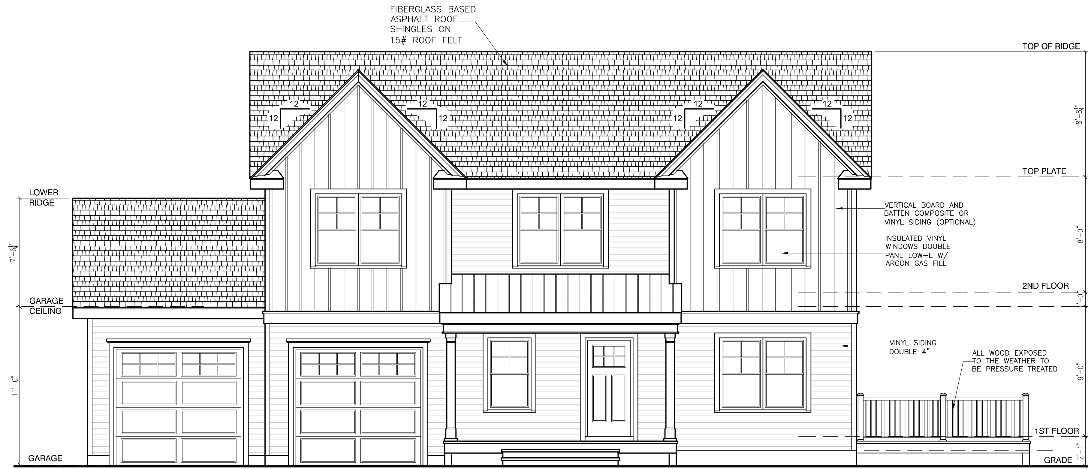
FRONT ELEVATION SCALE 1/4" = 1'-0"
